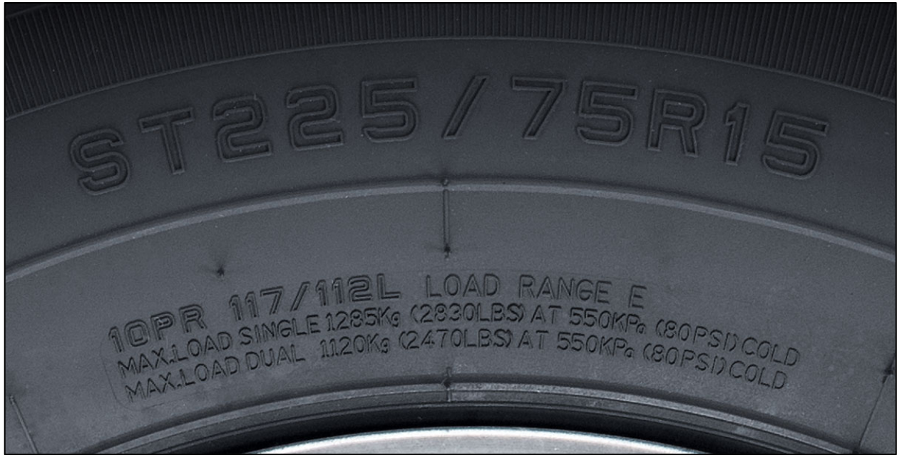
Above: Typical tire sidewall, showing tire type (ST), width (225mm), aspect ratio (75), radial (R), and rim size (15"). Note that it is a Load Range E, with a maximum single tire load of 2,830 lbs at 80 psi cold.
